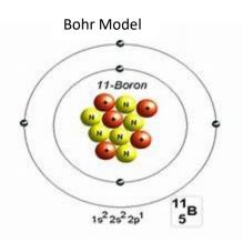
Two is the maximum number of electrons that fit in the first ring (shell, or energy level) and up to eight electrons fit in the second so we have two rings to fit the 5 electrons that this Boron atom has.
